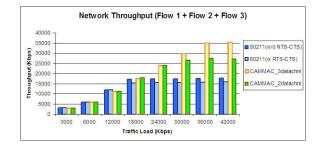
Fig. 4: Throughput comparision: CAMMAC vs 802.11 MAC.
